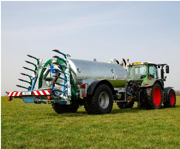
Picture 4: the UP folds compactly behind the tanker
